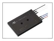
ACP's Coarse Wavelength Division Multiplexer (CWDM) utilizes thin film coating technology and proprietary design of non-flux metal bonding micro optics packaging. It provides low insertion loss, high channel isolation, wide pass band, low temperature sensitivity and epoxy free optical path .
